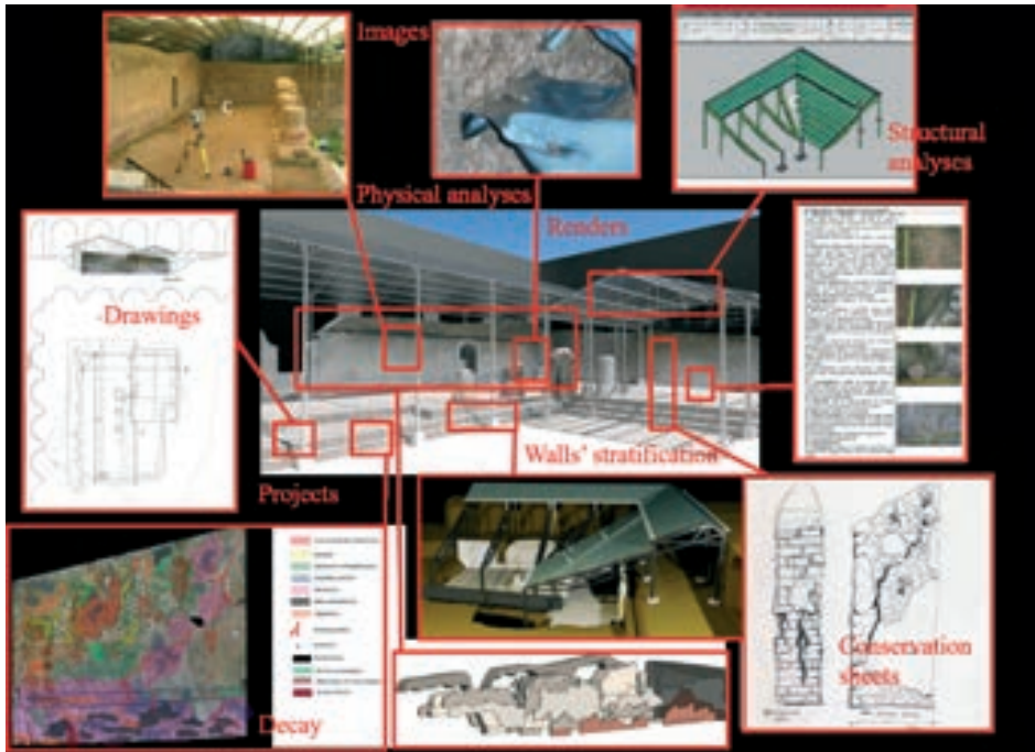
Figure 10. The BIM model meets the archaeological heritage, containing drawings, ad-hoc conservation sheets, structural analyses, photos, material analyses, walls' stratification, and more.
