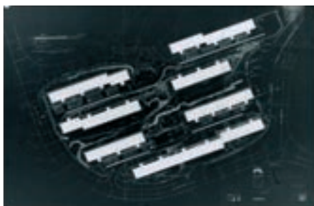
Figure 40 - Layout in which the bands of buildings are parallel and spaced equally to allow assembly with the same crane on a single trajectory. Source: Reaes Pinto/ICESA
