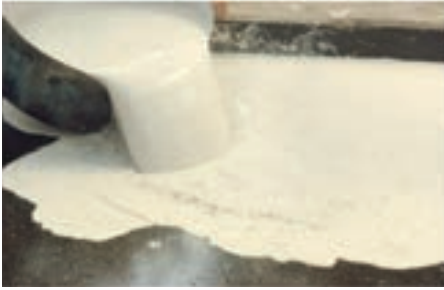
Figure 22 - Gypsum Plaster leaking into the mould. Source: Reaes Pinto/ICESA
