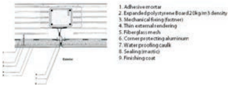
Figure 69 - Final solution – Rehabilitation of the external walls of the SAC and QM buildings with an external insulation composite system with rendering. Source: Reaes Pinto.
