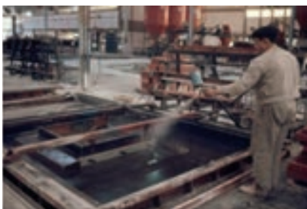
Figure 20 - General view of the factory – metallic horizontal moulds. Source: Reaes Pinto/ICESA
