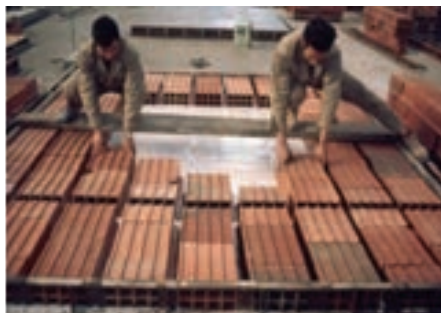
Figure 28 - Hydraulic Panel manufacturing mould with a finished partition wall. Source: Reaes Pinto/ ICESA 1968
