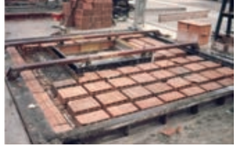
Figure 22 - Gypsum Plaster leaking into the mould. Source: Reaes Pinto/ICESA
