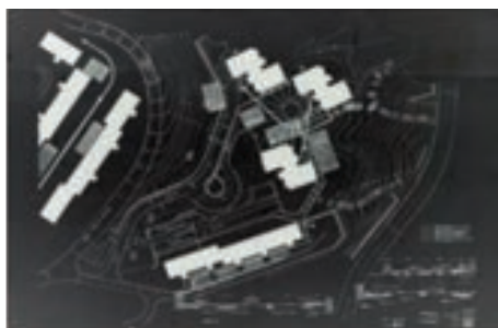
Figure 40 - Layout in which the bands of buildings are parallel and spaced equally to allow assembly with the same crane on a single trajectory. Source: Reaes Pinto/ICESA
