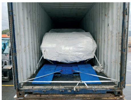
Figure 2. Container loaded with 2 boats and the platform
