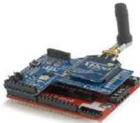
Figure 7: Arduino using Zigbee protocol [9]
