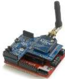
Figure 85: Arduino using Zigbee protocol [9]
